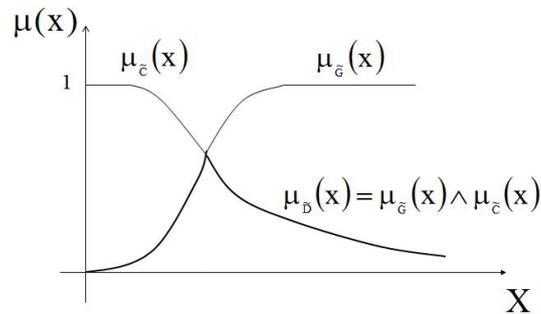
**Figure 2. Confluence between the goal and the constraint according to Bellmann and Zadeh’s criterion**
